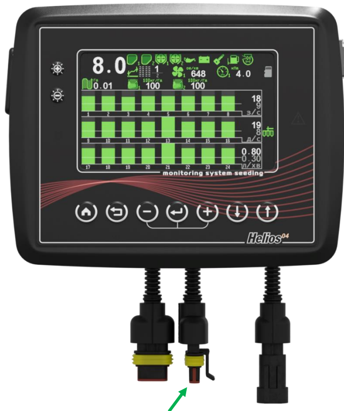
Figure 103 RS-485 communication harness connector
