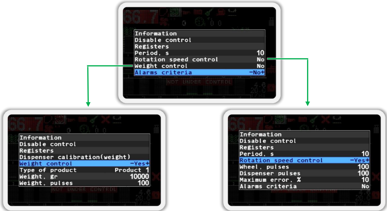
Figure 81 Parameters of the dispenser sensor
