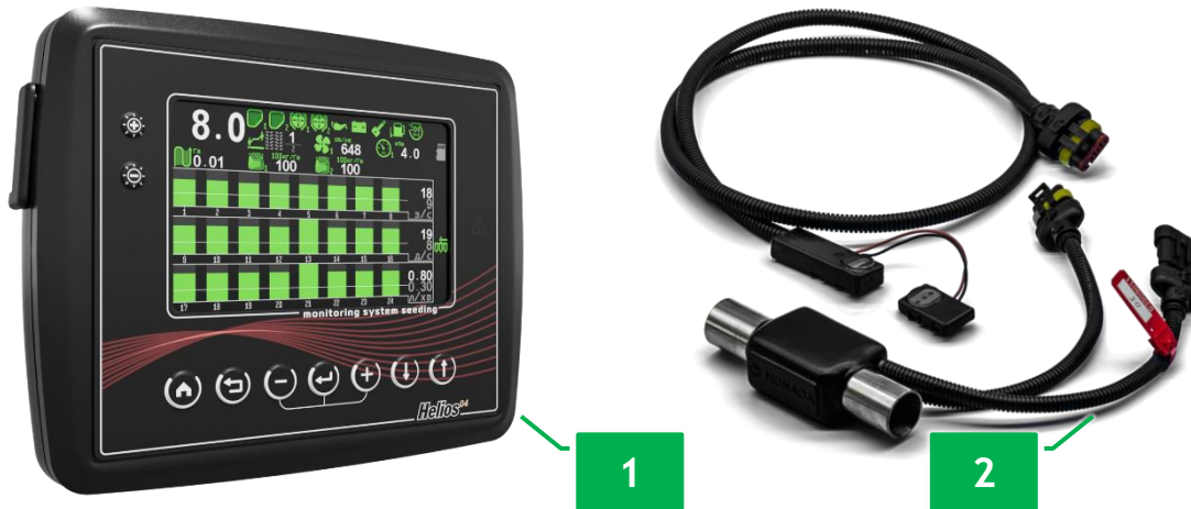
Figure 1 Operator panel and seed sensors
