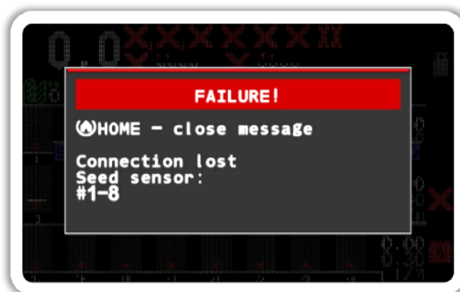
Figure 48 “Connection lost” alarm message window
