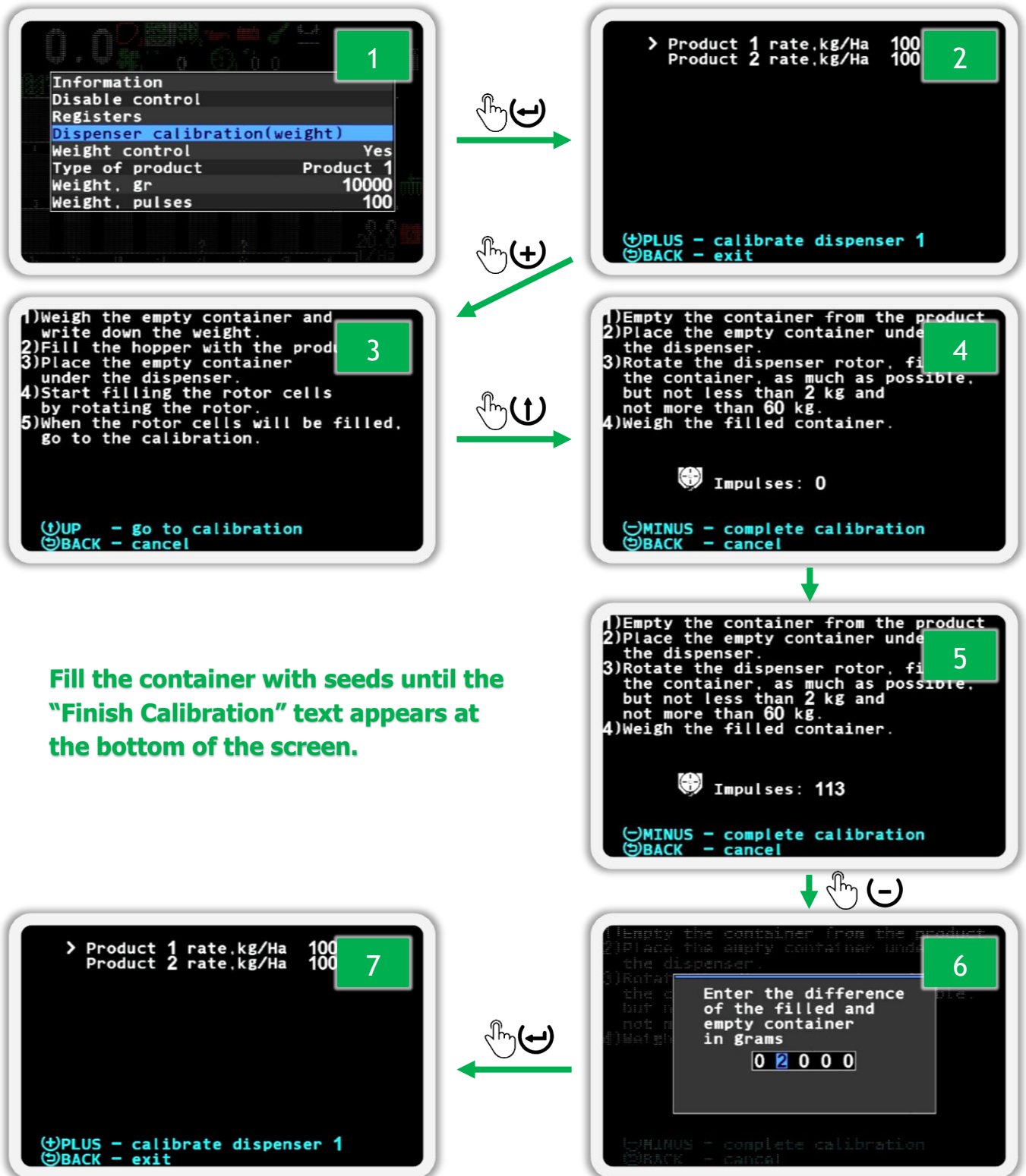
Figure 83 Calibrating the dispenser sensor for measuring the weight of product
