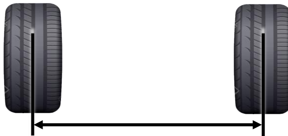
Figure 76 Measuring the distance between two wheels for the “Width, cm” parameter
