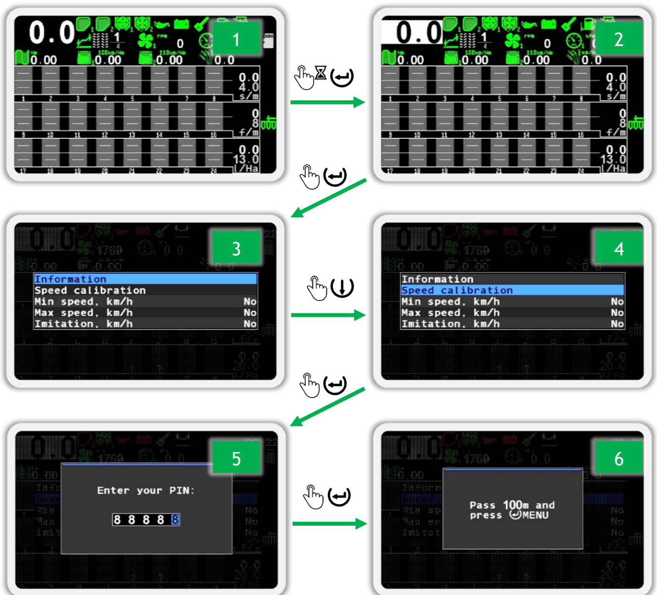
Figure 77 Starting calibration from the context menu of the sensor
