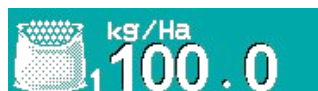
Figure 18 Indicator of the mass of product application by the central metering device
